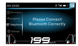
"Telephone" item will record all numbers that called in during this bluetooth connection. The records will be reseted when power off.
