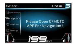
The instrument will display navigation interface when it activates in the cellphone.
